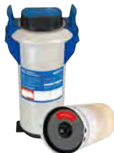
OS0803 PURITY 1200 EXTRA filter system with TOTAL demineralisation including filter cartridge. Connections: inlet G1"- outlet G3/4" Min./max inlet pressure: 2-6 bar Working temperature 4°-60°C Capacity: 5.000 l at 10° KH
