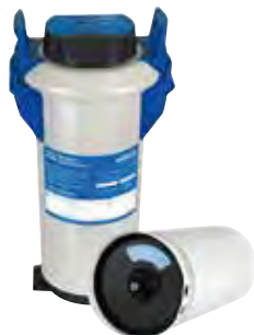
OS0801 PURITY 1200 CLEAN filter system with PARTIAL demineralisation including filter cartridge. Connections: inlet G1"- outlet G3/4" Min./max inlet pressure: 2-6 bar Working temperature 4°-60°C Capacity: 13.000 l at 10° KH
